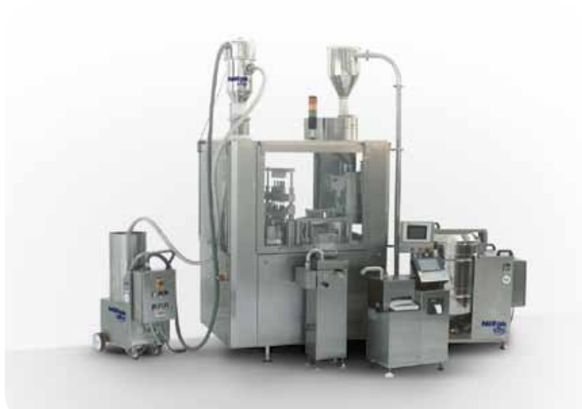
Pneumatic conveyor (left) and capsule pusher (right), in a pharmaceutical company
